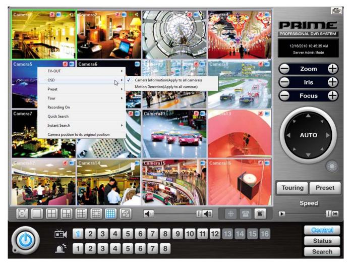
**Note:** One right mouse click can be a very useful tool. Manual TV-out and OSD setup can be done. Additionally, instant recording can start by one click.
