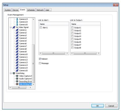
The same identical concepts and methods as "Input" are applied to "Disk Writing Failed" When "Disk Writing Failed" is occurred, it is linking to Alert and Output.
