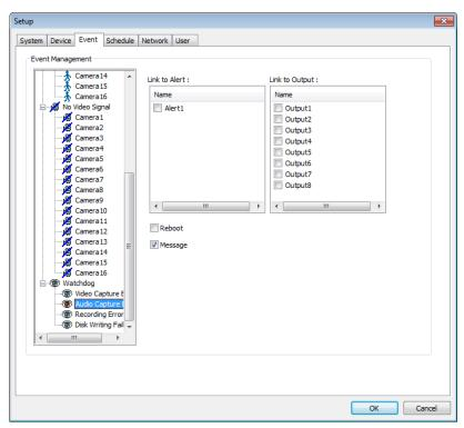
The same identical concepts and methods as "Input" are applied to "Audio Capture Error". When "Audio Capture Error" is occurred, it is linking to Alert and Output.
