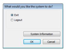
To end Prime DVR system, select "Exit" and type in password. Press OK button to continue.
