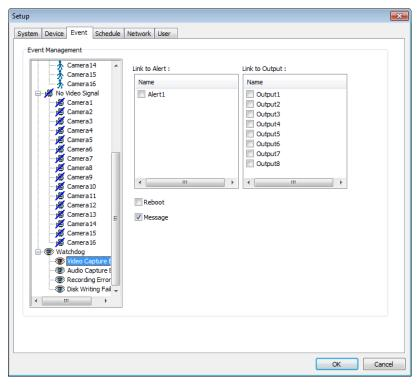
The same identical concepts and methods as "Input" are applied to "Watchdog". When "Video Capture Error" is occurred, it is linking to Alert and Output. User can link the event to Reboot, Message on DVR.
