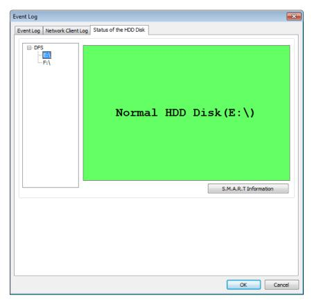
Every 5 hour DVR checks the status of HDD and shows its condition with different colors. Green: okay Yellow: Faulty is going on. Red: Completely fault.
