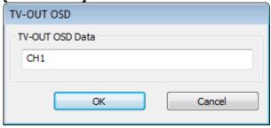
Camera name of TV out can be changed by TV-OUT OSD menu. Input camera name and press OK button to continue.
