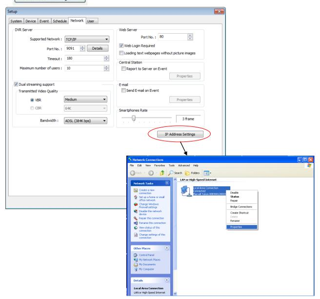
Click right mouse and select Properties for IP setup for DVR's network functions.
