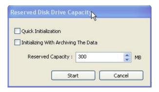
Selecting "Quick Initialization" will lead to the initialization of entire disk capacity added. Otherwise, put in desirable number to initialize. Note that the number can not exceed total capacity added. Initializing With Archiving the Data: This is to increase DFS storage by taking additional space from the current "Reserved Capacity". So new value for "Reserved Capacity" can not exceed the current one. Minimum 300MB is recommended for DVR performance.
