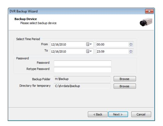
**Select Time Period :** Specify time period for backup. The minimum period for backup is 1 minute. If password is set, viewing backup data will be possible only when it is typed in.
