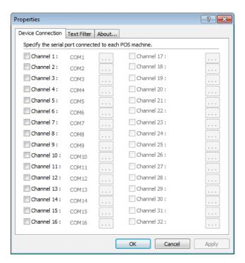
Device Connection: Select camera(s) and a comport connected with POS system(s)
