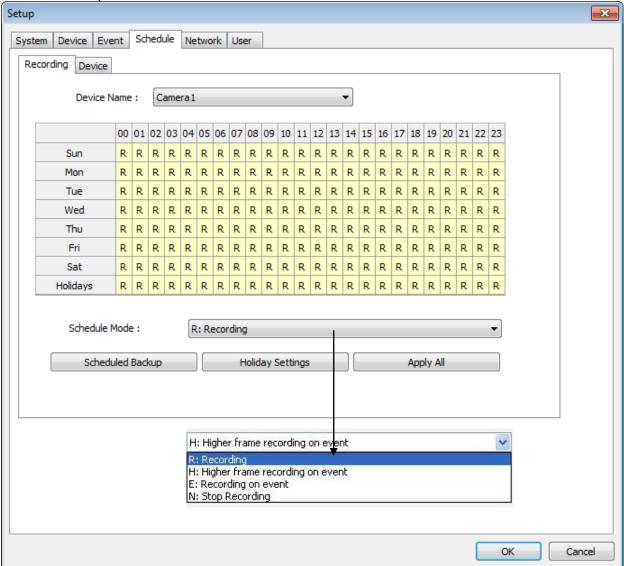
Each camera can have different recording options; scheduled recording by time & day and selective recording.
