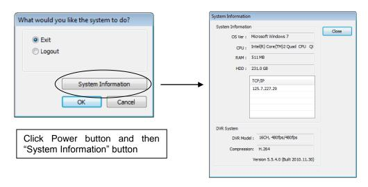
Click on System Information to see DVR system information, such as OS version, CPU, RAM, HDD, IP address, DVR model and DVR software.
