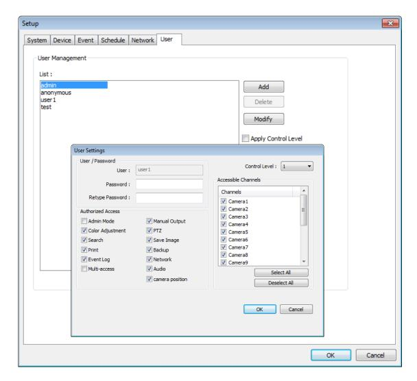
**Authorized Access:** If it checked, functions will be allowed to access remotely. **Accessible Channels:** If it checked, channels will be allowed to view remotely.
