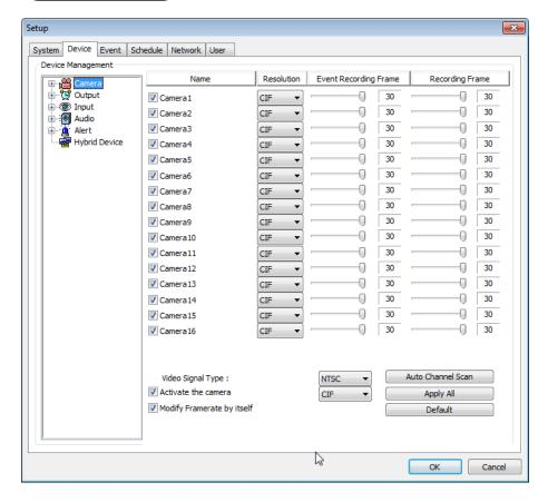
Device sub-screen is divided into 5 different setup categories; Camera, Output, Input, Audio Alert and Hybrid Device. (Hybrid Device category will be added by install hybrid driver. To integrate Hybrid device on 5.5.X.0 refer to page 52. "Hybrid Device")
