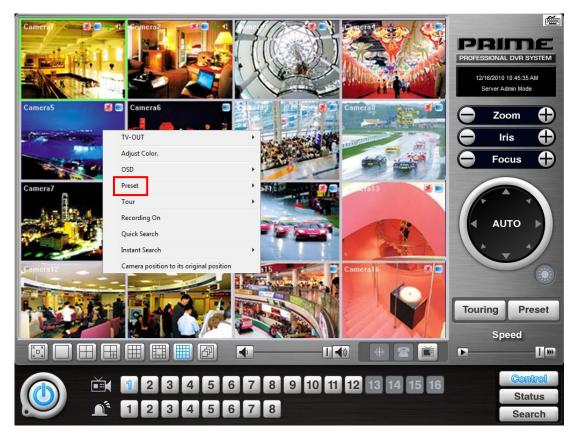
"Preset" is a function that enables a camera to move from one position to another automatically.
