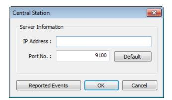
Type in the IP address of Central Station Server (Client with Static IP) and click on "Reported Events" for more setup.
