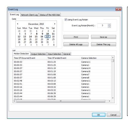
**Using Event Log Retain:** Event log can be saved into DVR automatically from 1 to 12 months and its default setting is 3 months. It is to avoid overloading of event log.
