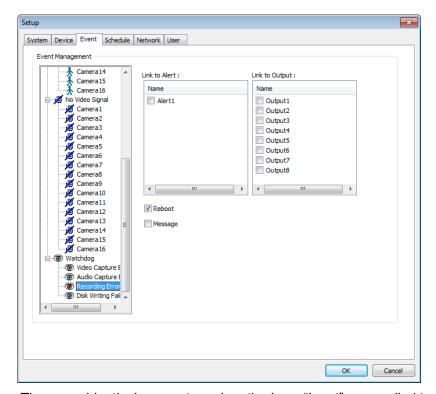
The same identical concepts and methods as "Input" are applied to "Recording Error". When "Recording Error" is occurred, it is linking to Alert and Output. User can link the event to Reboot, Message on DVR.
