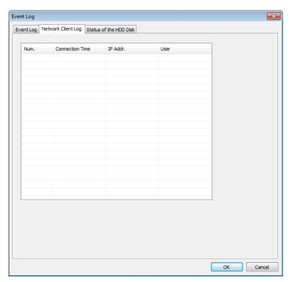
**Network Client Log:** Remote login records will be also kept on DVR server. Checking accessed network user, connected time and IP address are available.
