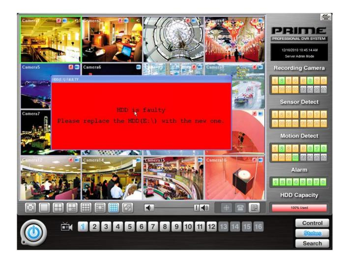
If HDD is completely fault, POPUP menu as above will be shown. It rests till the system shuts down, and it shuts down below message will be appeared.
