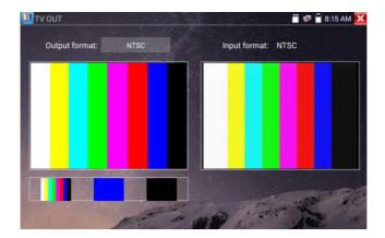
**BNC loop test:** Tester can send and receive color bar generator through the tester's "video out and video in" port, it is for testing transmission channels, such as video Optical, video cables etc. The tester "VIDEO OUT" port to connect optical terminal's sending port, and "VIDEO IN" Port to optical terminal's connect its receiving port.
