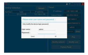
**Factory reset setting:** Camera will be soft reset, and the device's user name, password and network set be saved. Other settings information is factory reset.
