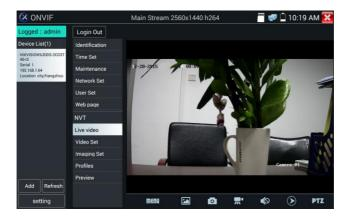
**ONVIF PTZ control:** Tap the image in the direction you want the PTZ camera to move. Tap the left side of the image to move left, right to go right, up to go up and down to go down. Compatible IP PTZ cameras will rotate accordingly. PTZ rotation direction is displayed on top left corner of the image.
