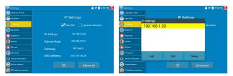
After setting an advanced IP address (refer to the photos above), the unit can test two network segments (192.168.5.0) and (192.168.1.0).
