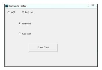
Tester as Client, tester's IP address is:192.168.0.238. The Server and the Client are at the same network segment, but with different IP address. Input Server's IP address 192.168.0.39 in the tester and click "Start" to test network bandwidth.
