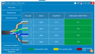
Single test: Test cable status, length and attenuation.
