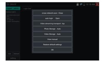
Across network segments scan: After open this function, enter "Setting - IP Settings - Advanced" to add other network segments IP, Rapid ONVIF function can across network segments to scan camera's IP.
