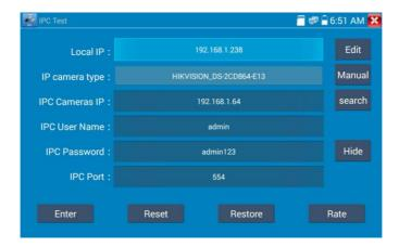
**Local IP**: This is the tester's IP address. Click "Edit" to enter "IP setting" and change the tester's IP address settings.
