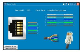
Test LAN cable or telephone cable.
