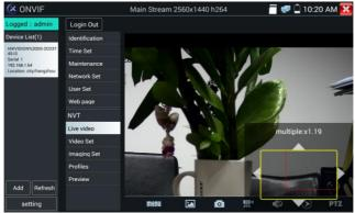
When the image is enlarged, if not operate on touch screen, it can operate by the keyboard, press the key (WIDE-) to zoom out , press upward and downward key to move image.
