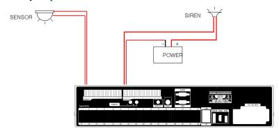
**Sensor In**: Connect the sensors. The sensor are composed of both signal and ground terminals, with a voltage difference of 5V. In the case that the sensor used for input is of the N/O (Normal Open) type, when the voltage difference between the signal and ground falls to 0V (short), the NVR can use this as a trigger to start alarm/sensor based recording.
