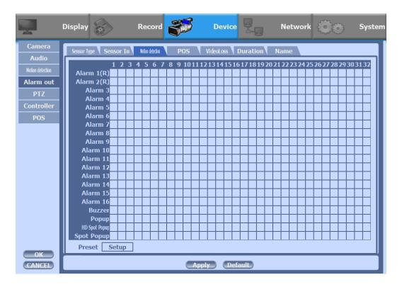
• Also you can choose more than one action. Furthermore you can set the preset position number by motion detection. If you push the 'setup' you can see the preset screen.
