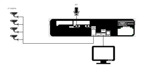
Connect cameras to POE PORTS by channels. Connect microphone (AMP) to AUDIO IN by channels. Connect VGA OUT to VIDEO IN of monitor. Connect HD output to HD Monitor. Connect AUDIO OUT to AUDIO IN of monitor (or speaker).
