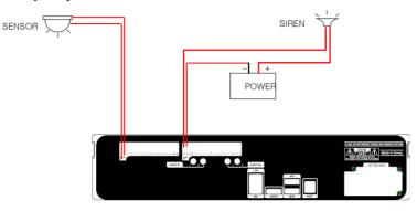
**Sensor In** : Connect the sensors. The sensor are composed of both signal and ground terminals, with a voltage difference of 5V. In the case that the sensor used for input is of the N/O (Normal Open) type, when the voltage difference between the signal and ground falls to 0V (short), the NVR can use this as a trigger to start alarm/sensor based recording.
