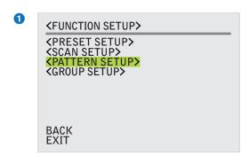
Select '<PATTERN SETUP>' and press the 'NEAR' key
