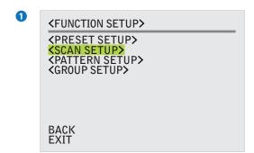
Select '<SCAN SETUP>' and press the 'NEAR' key
