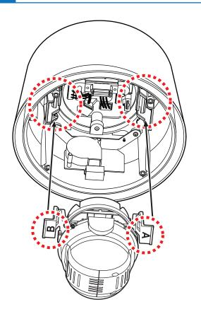
Plug the connector of cable from junction box into properly. After checking the orientation of one touch connector in the upper housing, press the PTZ mechanism into hook in the upper housing.
