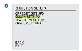
Select '<SCAN SETUP>' and press the 'NEAR' key
