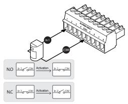
It is noted that short circuit between GND and Input pin means alarm activation.
