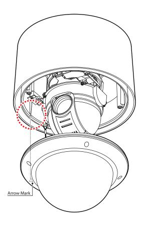
Olose the dome cover. Care must be taken to locate dome cover by matching the 'Arrow Mark'.
