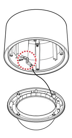
8 Make sure that the dome cover is connected firmly to the safety wire.
