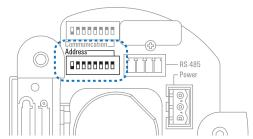
ID number of camera is set using binary number. The example is shown below.
