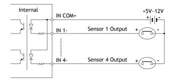
Before connecting sensors, check driving voltage and output signal type of the sensor. Since output signal types of the sensors are divided into Open Collector and Voltage Output type in general, the cabling must be done properly after considering these typed. Also, the sensor type, i.e. "Normal Open" or "Normal Close" in Dip switch in main body of camera must be set properly.
