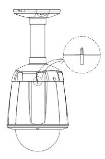
(5) Turn main body on its axis in CW(Clockwise) direction and, after assembling them, screw main body to Ceiling Mount Bracket to protect them from separation by vibration or others.
