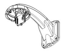
4 Line up the mold lines and assemble main body
