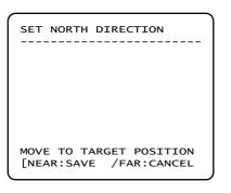
Set North to assign compass direction as criteria. Move camera and press **NEAR** button to save.
