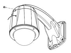
(6) In case of using pipe, use the hole located on lower side of Wall Mount Bracket to fix pipe.
