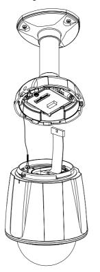
② Wire cables to terminal blocks on the PCB in Ceiling Mount Bracket.
