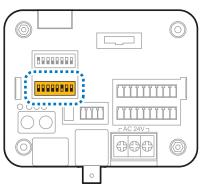
ID number of camera is set using binary number. The example is shown below.
