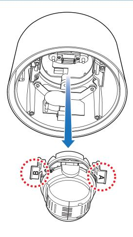
(5) You have to detach the PTZ mechanism from the upper housing to plug the connector of cable. When detach PTZ mechanism, pressing down and holding up the black handles in both sides of PTZ mechanism.
