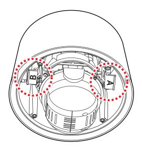
**3** To lock the PTZ mechanism to the upper housing, press the two black handles till it sounds snap.
