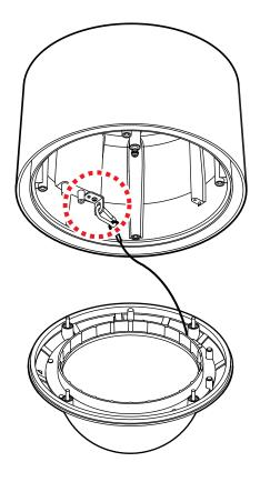
**3** Connect the dome satety wire into the connectors in the upper housing.
