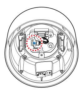
7 Plug the main cable into the main connector in the upper housing and press the main cable till it sounds snap to lock.
