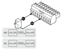
It is noted that short circuit between GND and Input pin means alarm activation.
