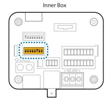
ID number of camera is set using binary number. The example is shown below.
