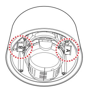
**8** To lock the PTZ mechanism to the upper housing, press the two black handles till it sounds snap.
