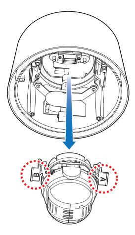
S You have to detach the PTZ mechanism from the upper housing to plug the connector of cable. When detach PTZ mechanism, pressing down and holding up the black handles in both sides of PTZ mechanism.
