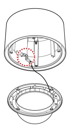
8 Connect the dome satety wire into the connectors in the upper housing.
