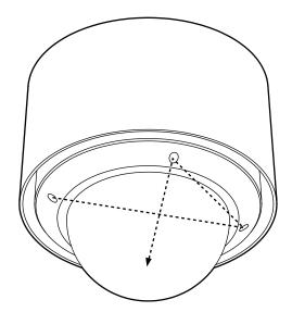
① Tighten four screws on the dome cover in sequence as shown in the picture.
