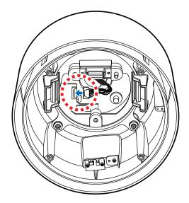
Plug the main cable into the main connector in the upper housing and press the main cable till it sounds snap to lock.
