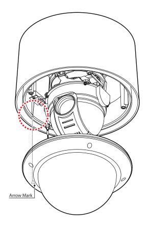
Olose the dome cover. Care must be taken to locate dome cover by matching the 'Arrow Mark'.
