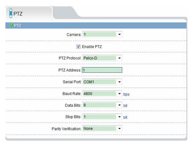
When connect external PTZ, you can configured PTZ agreement address, bit rate, data bit.
