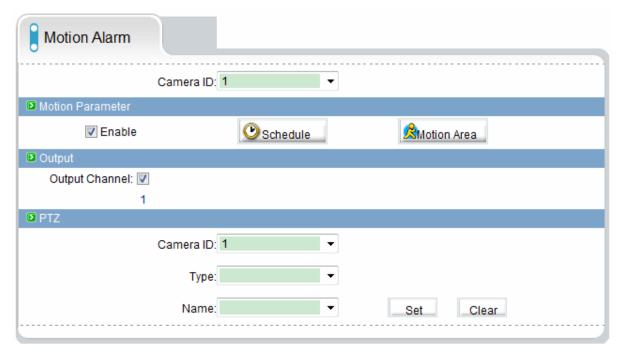
Options the camera that need to configure ID number, can be configured to detect movement of the camera to trigger the alarm when the linkage. Including whether the alarm output and whether or not such as the opening of PTZ.
