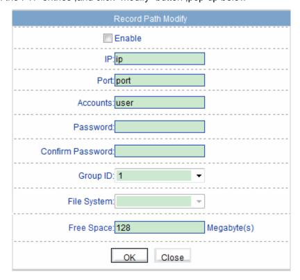
Set the right FTP IP address, port, account number and password, click the "opening" button, equipment video recording can directly record to the FTP.
