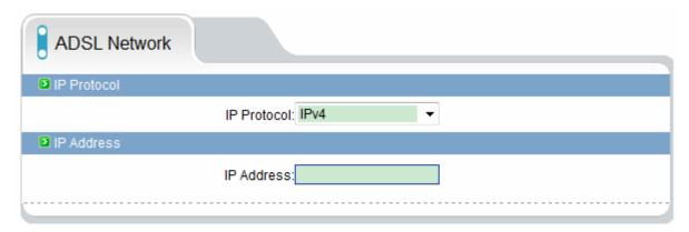
When the user set "Network Service" "PPPoE parameters", after the success of dial-up equipment, Equipment's WAN network IP address will appear in the page.
