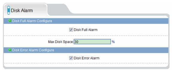
Disk Alert configuration including: disk error alarm and disk full alarm. Disk alarm will be recorded in the alarm log.
