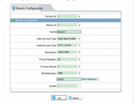
Each device can be configured for different video stream; each device can be configured with up to three different video streams.
