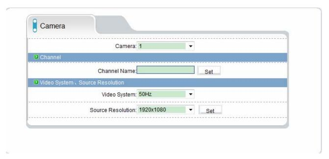
Camera name: option the camera that need to set up, you can set the camera both English and Chinese name. Name of the success of the camera settings will be displayed in real-time monitoring--Device list.
