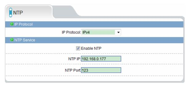
NTP: Network Time Protocol. Host can automatically adjust the clock of the computer and connect sync. Click "Apply" button and then automatically adjust the time, In addition, 12 o'clock everyday, the automatic adjustment of service start.
