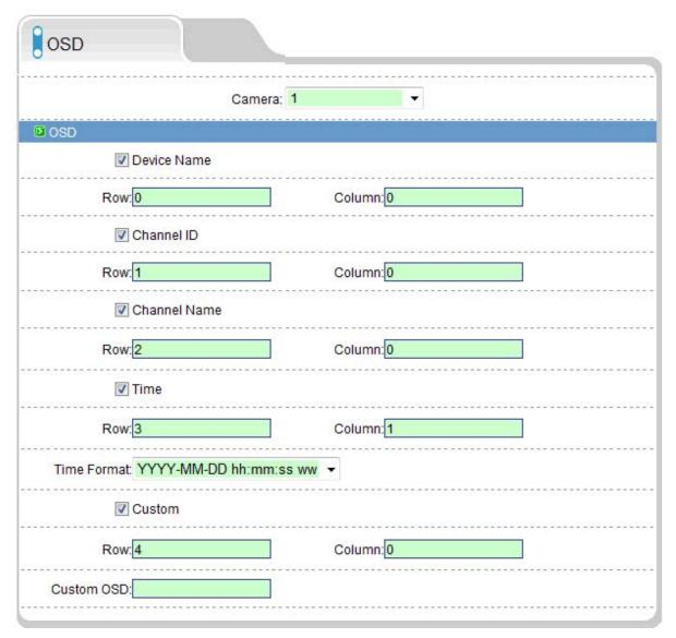
Respectively for different resolutions of network device to set OSD parameters, including: device name, channel number, channel name, time and custom OSD. OSD settings will be held at the image on the overlay.
