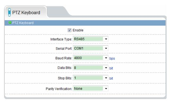
When connect PTZ keyboard ,you can configure interface type serial ports bit rate data bit.
