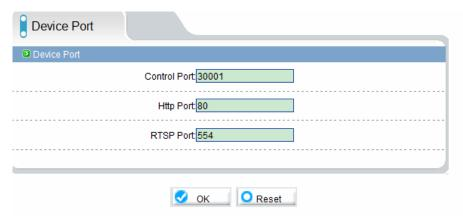
Control port: The default is 30001, including the parameters of reading and writing, PTZ control are both through this port to control;
