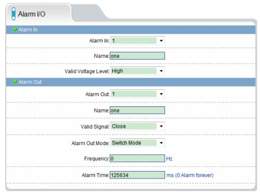
Alarm input: Select the alarm input configuration ID, the alarm can be chose the effective level. Effective level include: high and low two options. When you select high effective input port when access to high level alarm that is triggered by alarm signals, When you select low effective input port when the alarm signal that is triggered off high alert.
