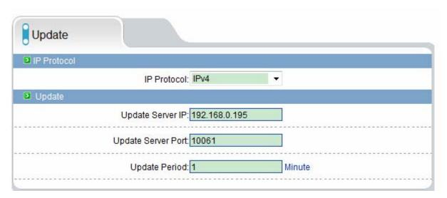
You can be set to upgrade the server IP address and port number as well as parameters such as the upgrade cycle.
