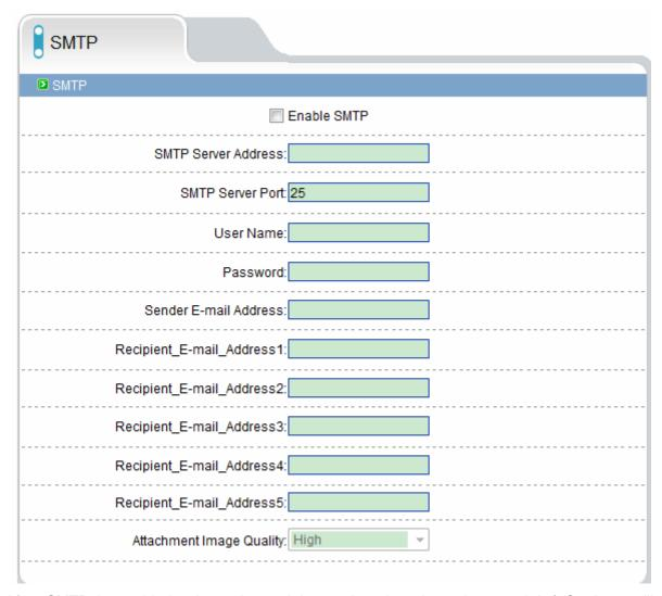
After SMTP is enabled, when triggered by motion detection, alarm and I / O alarm will be
