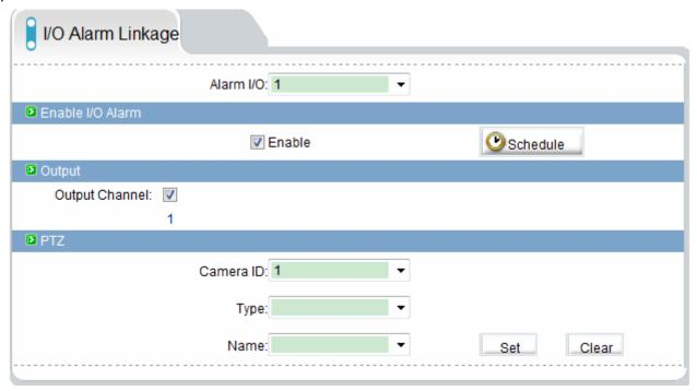
Options need to configure the alarm I/O of the ID number, can be configured in the Alarm I/O trigger the alarm when the linkage. Including whether the alarm output and whether or not such as the opening of PTZ.
