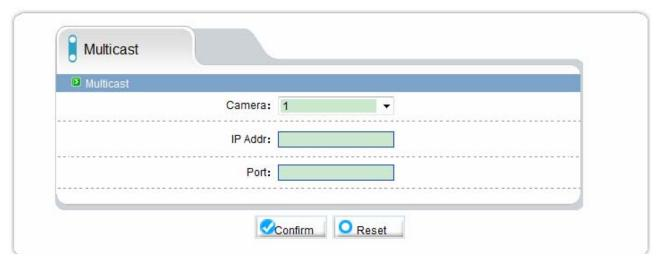
This function can make a single flow provide more network receivers.
