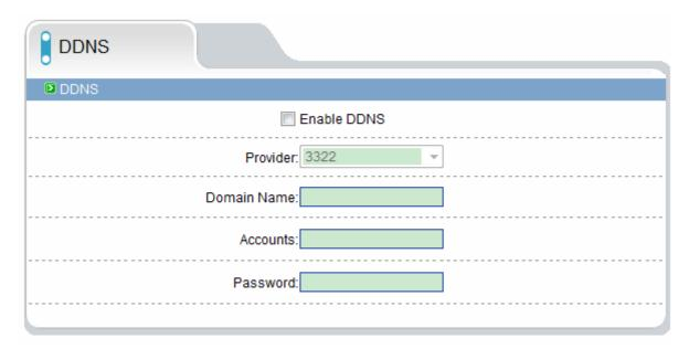
DDNS: Dynamic domain Name service: It is better to register a domain for avoiding input IP address, as IP address is difficult to remember. It is necessary to get a PC with stable IP address in Internet, and domain name service software need to be run on the PC.(The PC will be DDNS)
