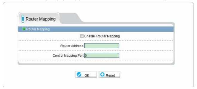
The router address :fill the router WAN address, support filling in domain name address, such as test.gicp.net。
