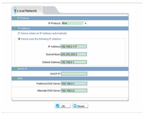
It Can set the network IP camera address, subnet mask, gateway, DNS and other network parameters, If it is used in local area network You should be careful that not to set up the internal LAN IP address and computer IP address conflict .If you want to modify equipment IP protocol, the client must restart the selection of the corresponding IP protocol registry.
