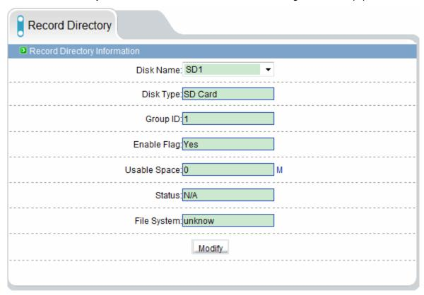
**1. SD** card: SD Card: Click on the SD card entry, click on the button "modify", you can format the SD card, the following figure:
