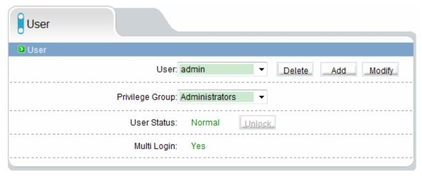
You can add, modify, delete a user, but the default user admin can to be deleted. The default user can unlock the customers which input wrong password for many times.
