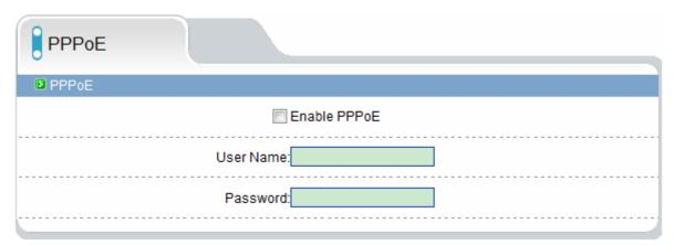
PPPoE: Network Camera support agreement based on the PPPoE WAN access. Through the client software is set up correctly PPPoE username and password, after every time you start Network Camera, PPPoE mode automatically establish a network connection, after the success of the network camera to obtain the dynamic WAN IP address.
