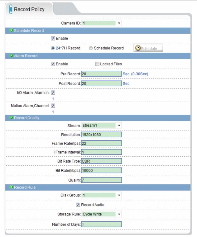
Need to set up the camera to choose ID, you can set the camera to record the quality of SD cards, including: resolution, frame rate, bit-stream parameters.
