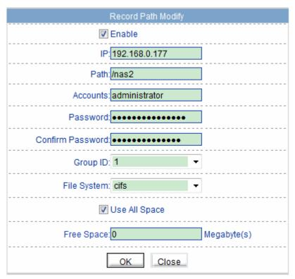
Set the correct IP address of the NAS, path, username and password, Click enabled, you can record video directly to a device on the NAS.
