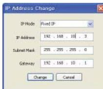
It is possible to change IP address of a server which has IP address of different subnet.
