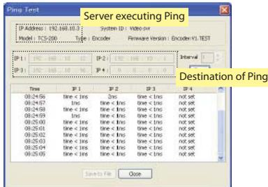
Ping test is useful for checking if one or more remote systems are reachable from a server. Up to 4 systems can be registered as the targets of Ping test, which makes it possible to identify the hop(segment of network) where network failure may happen. For example, local router, remote router and remote Encoder can be pinged from a Decoder simultaneously.
