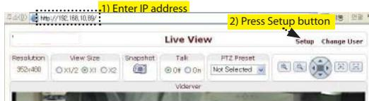
The configurations are grouped into 8 categories: System, Video, Audio, Network, Serial, Event, Preset and User. Any configuration changes are not applied until Apply button is pressed. Leaving the page without pressing Apply button, changes in the page will be discarded.
