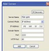
If the server is registered on DDNS server, domain name can be used instead of IP address. When the IP address of the server is forgotten, it is possible to find the IP address of the server with IP Discovery function. (Please refer to IP Discovery section).
