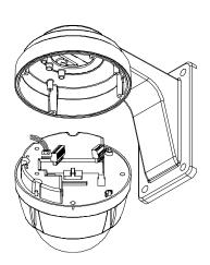
$\ \ \,$  Screw main unit to wall mount bracket with 4  $\ \ \,$  Detach protection vinyl from dome cove. screws.
