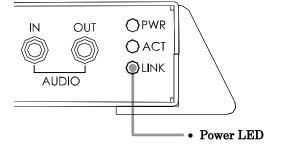
This red light becomes illuminated when 12V DC power is supplied to the unit. This indicator should always be lit when in use. If it is not lit or flashes when power is supplied, the Video Server is not operating properly.
