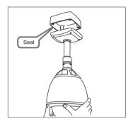
1b - pendent option. After making all the connections to the PCB, raise the dome assembly to the junction box, connect the dome cable to the PCB and fix with the four screws.
