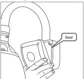
1a - wall bracket option. After making all the connections to the PCB, fit the junction box cover with the four screws.
