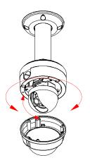
⑤ Fix the dome cover by screwing 3 screws ⑥ Remove protection vinyl from the clear dome provided.
