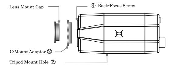
① Lens Mount Cap Be sure to plug the lens mount cap when the lens is not
