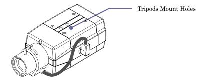
2 Mount the camera on the proper mounting bracket.
