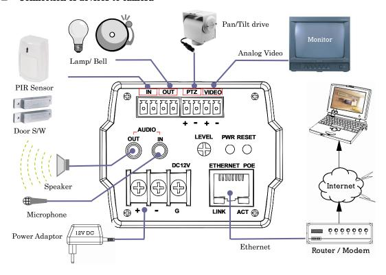
Connect the video output of the camera to the video input of a monitor or other equipment. When using a "loop through" connection of two or more monitors, set the  $75\Omega$  switch of only the final monitor to 'On'. Determine the type of cable according to the distance of the connected equipment.
