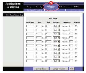
4) Input port numbers in " Port Range" as below and click " Save Setting" button. Both of Web Server Port and Video Server Port should be added. The example is as below.
