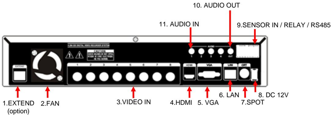
1. **EXTEND (option)** : Connect EXTEND FTP cable to VGA or HDMI Receiver
