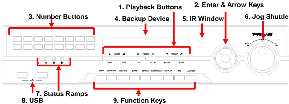
**1. Playback buttons** : It will be used on playback. If you press these buttons in live mode, it will be automatically changed to the Instant Play mode. ‘Stop’ button changes from the play mode to the live mode.
